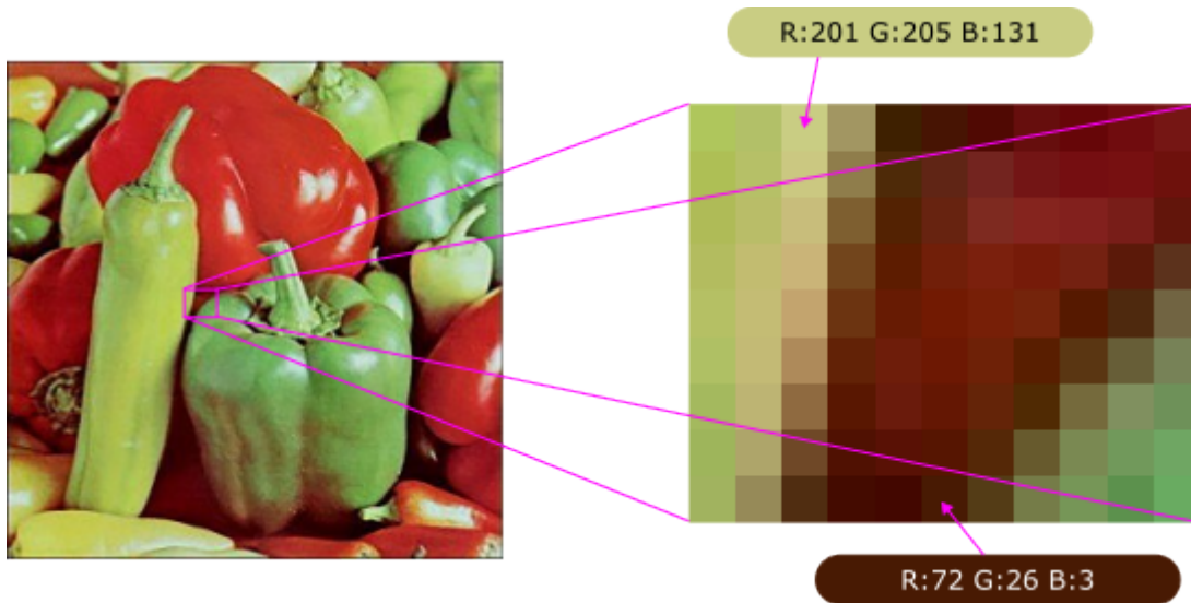
Fig. 2: Computerized image organized using pixels. A color image usually requires RGB brightness values to represent the final pixel color.
