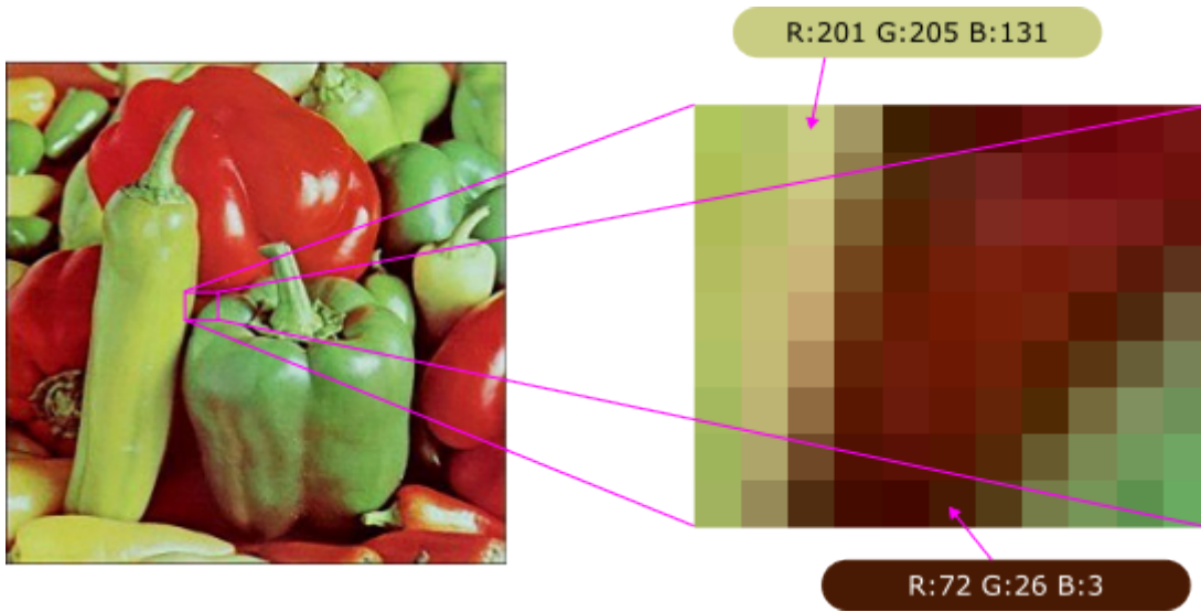
Fig. 2: Computerized image organized using pixels. A color image usually requires RGB brightness values to represent the final pixel color.
